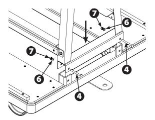
3. Place cross members between A-Frame ends as shown. Fasten in place to flatbar gussets using 3/8" x 1-1/4" hex bolts, 3/8" flat washers and 3/8" Nylon lock nuts provided. Repeat for all 6 cross member pieces.
