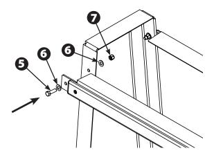
4. Tighten all 3/8" fasteners put in place during steps 3 and 4 using a socket.
